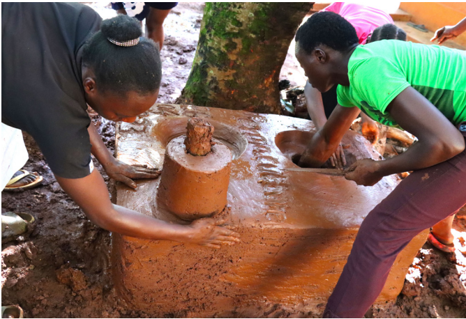
Hand-made Lorena stoves are low-cost, fuel-saving cookstoves, made of sand and clay.
